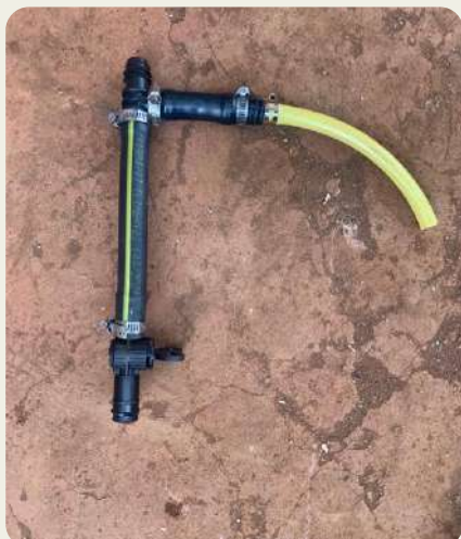
Connect the T-connector. It should be lower than the stove's table
