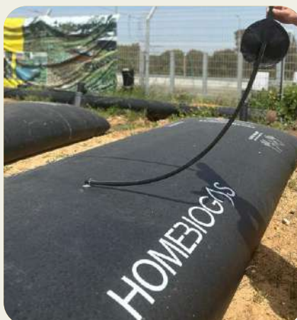
Add the outlet cover to the gas pipe
