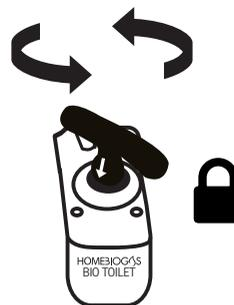
**DESPUÉS DEL USO: EMPUJE LA MANIJA TOTALMENTE HACIA ABAJO Y GIRE HASTA QUE SE BLOQUEE**
