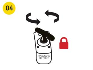
AFTER USE- PUSH THE HANDLE DOWN FULLY, AND ROTATE UNTIL LOCKED
